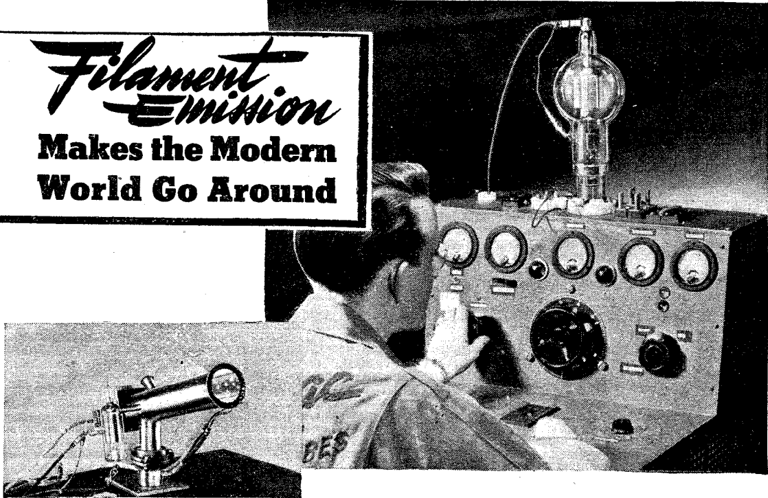
Close observation of the flow of electrons from a heated filament is made possible with this Electron Microscope. This instrument, designed and constructed in the Eimac laboratories, virtually gives a motion picture projection of the electron movement.
