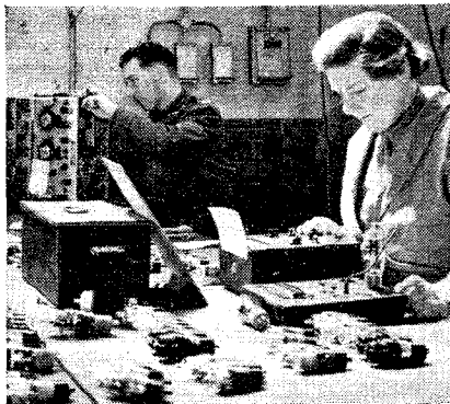
A TRAINEE A.T.S. wireless mechanic testing valves in one of the repair bays of an R.A.O.C. wireless workshop.
